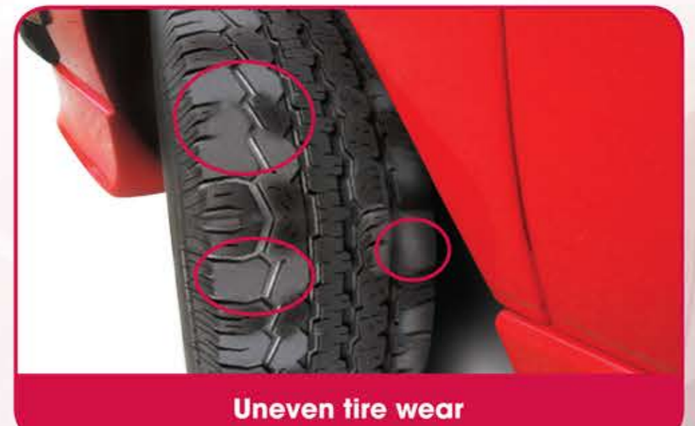
Uneven tire wear
